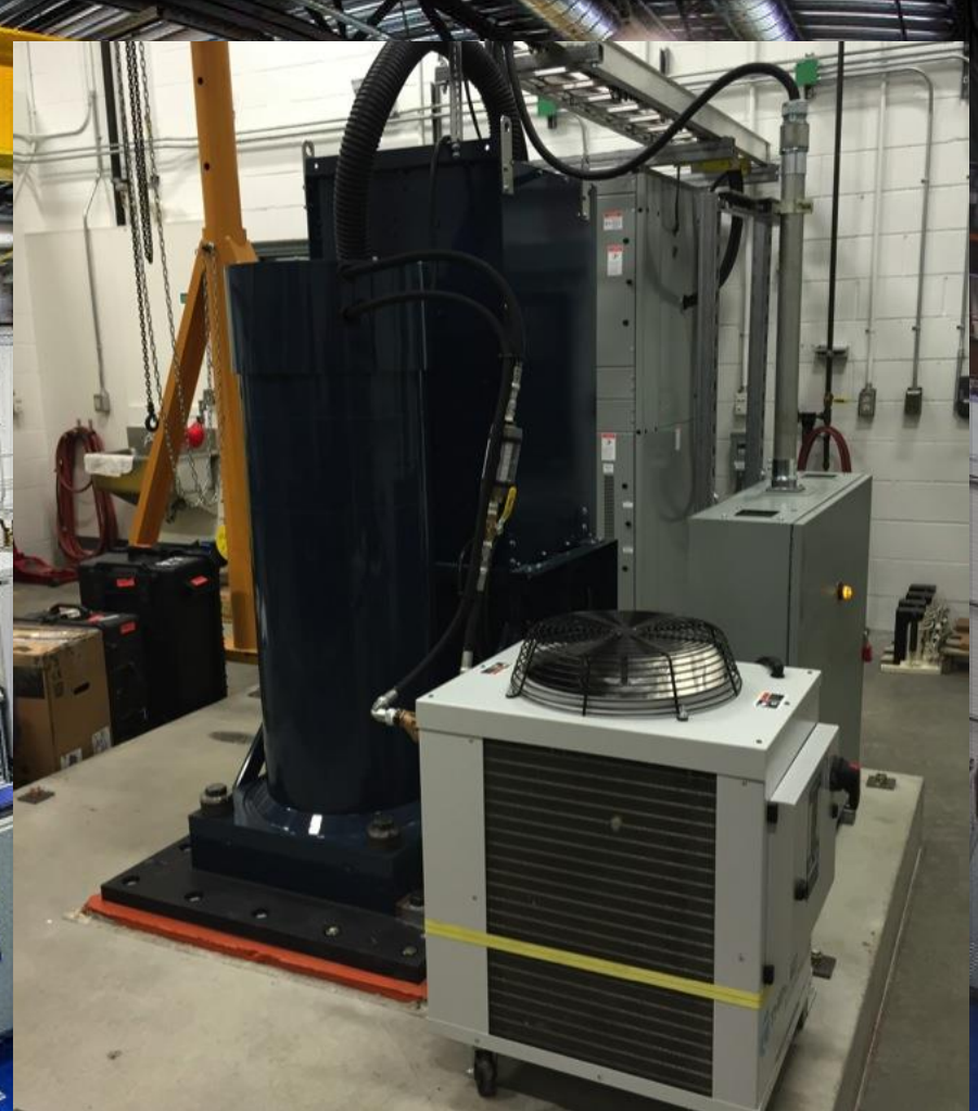
Williams flywheel testing for Hatch Engineering prior to installation at Raglan Mine
